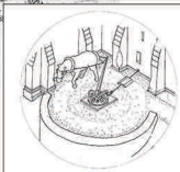
In the 19th century a platform was built for a horse-gin. The horse pulled on a shaft fixed to a pivot which rotated a crown wheel. That worked a machine (e.g. chaff cutter, turnip cutter) inside the barn.
